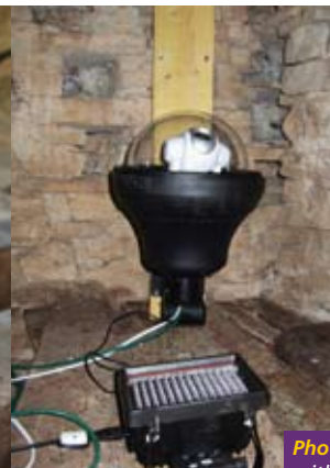
Photo 12 : Infrared projector of 140 leds of 3 mm (a widespread product).
